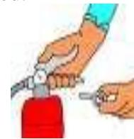
**AIM at the base of the fire:** Point the extinguisher hose/nozzle at the base of the fire.
